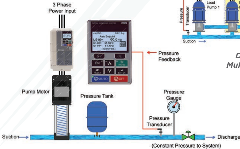
Simplex Pump System
