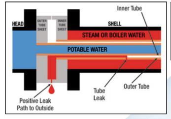
The SDW and WDW are made with inner and outer double tubes and double tube sheets that provide a positive leak path between the two fluids. This design prevents the cross-contamination of the potable water by the surrounding steam or treated boiler water.
