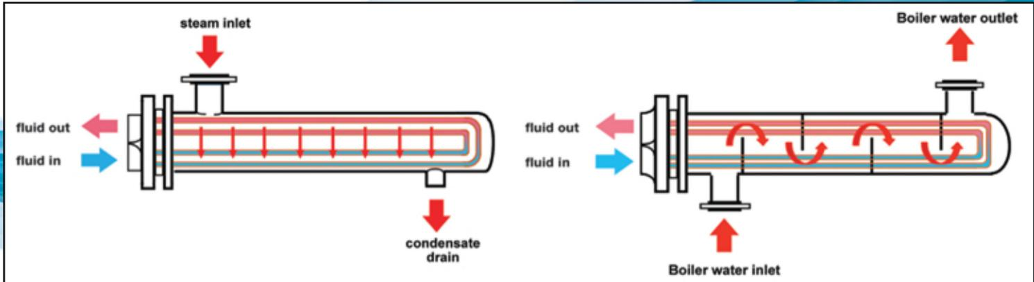
The S works by introducing steam (water vapor) into the shell where it naturally distributes across the outer tube surface and condenses and heats the water inside the tubes. The condensate exits through a drain in the shell. Tube supports carry the weight of the tubes and do not divert the steam.
