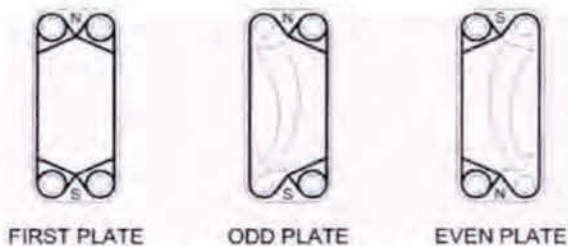
Figure 1.7 - Models Same-Side Flow • FLO FAB standard design
