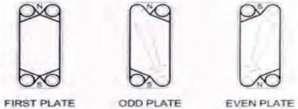
Figure 1.8 Models with Diagonal Flow • FLO FAB special designs
