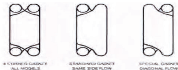
Figure 1.5 Types de joints
