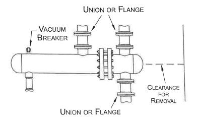
NOTE: LOOSEN UNIONS/FLANGES ON TUBESIDE HEADS PRIOR TO RETORQUING HEAD BOLTS.
