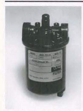
The 1A1 MODEL Cartridge Filter Housing is an all-metal, two-piece housing, featuring centerpost-type construction. The 1 Al Model has a maximum operating temperature and pressure of 125 psig at 200°F. The 1A1 Model Cartridge Filter Housing has flow rates to up to 6 Gallons Per Minute (GPM).
