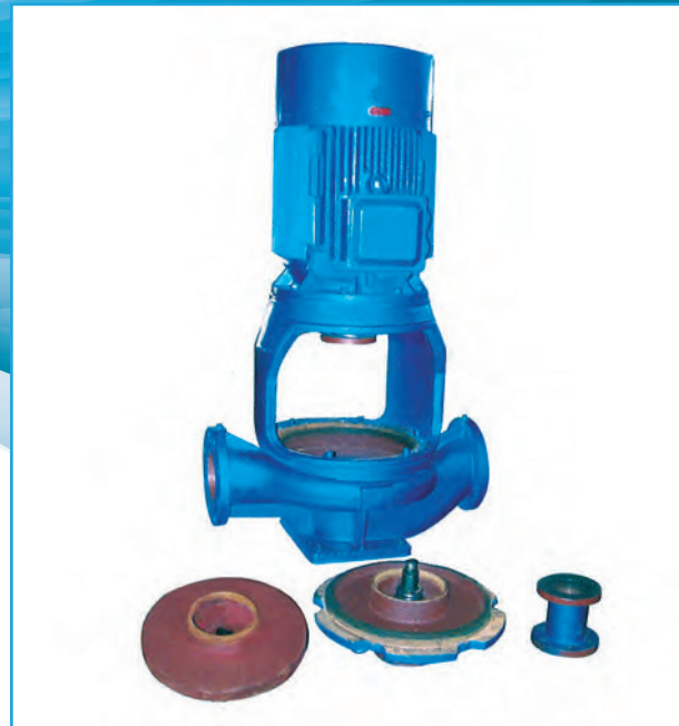
Repair the wearing parts when pump is disassembled, ready to be repaired or serviced
