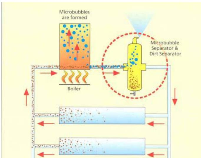
The threaded connection at the air vent outlet has been provided as a convenience for those wanting to pressure test the system with air prior to filling.
